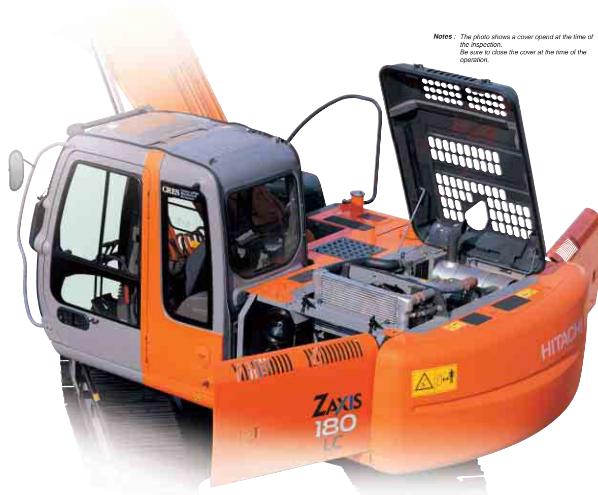
Water separator Engine oil filter Engine Oil Filter and Water Separator Positioned for Easy Access from Ground
