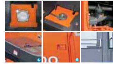
1 Fuel cap 2 Hydraulic fluid cap 3 Transmission fluid cap 4 Battery box 5 Side cover 6 Cab door
