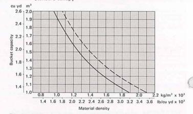
This guide will help you in selecting proper bucket size for material density and loader configurations. However, specific bucket size should only be determined after adding or subtracting all the tipping load changes due to specifications.
