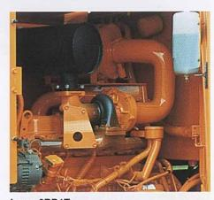
4-cycle, direct injection turbocharged diesel engine has high power to 85.8 kW (115 HP) and sharp torque rise for powerful operation.
