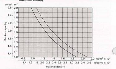
This guide will help you in selecting proper bucket size for material density and loader configurations. However, specific bucket size should only be determined after adding or subtracting all the tipping load changes due to specifications.
