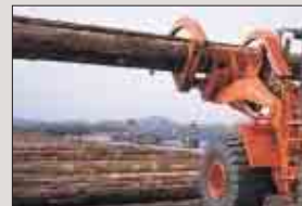
Log grapple This dedicated attachment allows the loader to handle logs and other round materials.
