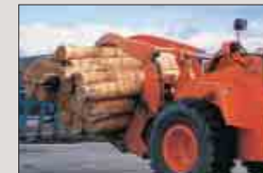
Lumber grapple Forks pick up the square material and the upper arm comes down to hold the load in place during transport.
