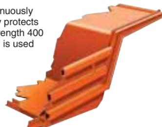
High strength 690 N/mm<sup>2</sup> (100 000 psi) alloy steel is also used for the canopy side members and floor stiffeners. The body is rubber cushioned on the frame.
