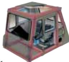
Double wall construction of 11 gauge inner and outer steel panels produces a more structurally sound cab. Foam rubber lining material along with foam rubber-backed carpeting and multiple layered floor mat act to absorb sound and control interior temperature.
