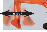
Arm piping is increased in diameter to reduce hydraulic loss (theoretically 7%) for speedy front operation.
