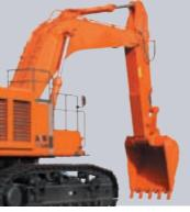
The arm and boom are strengthened by thickening and using stronger material.
