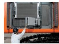
allow servicing from one side of the machine. This can significantly reduce servicing time and costs. The hood cover is reduced in weight and provided with a damper for easy opening and closing.
